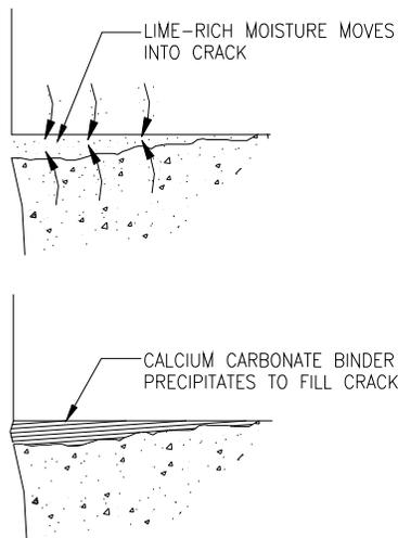
Figure 2. Lime in mortar provides autogenous healing capabilities – the ability to self-seal small cracks and voids.
