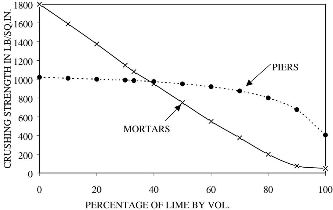
Figure 1. Mortar compressive strength has little effect on masonry assemblage strength except in extreme cases (adapted from Davey).
